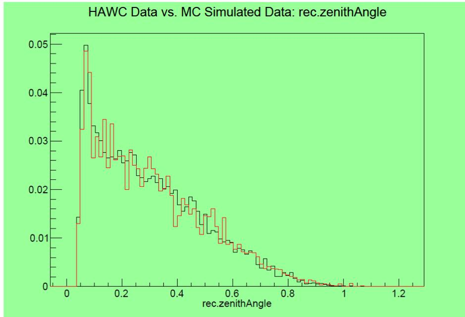
Figure 6: Comparison of zenith angle in actual vs. MC data (red = MC, black = actual)
