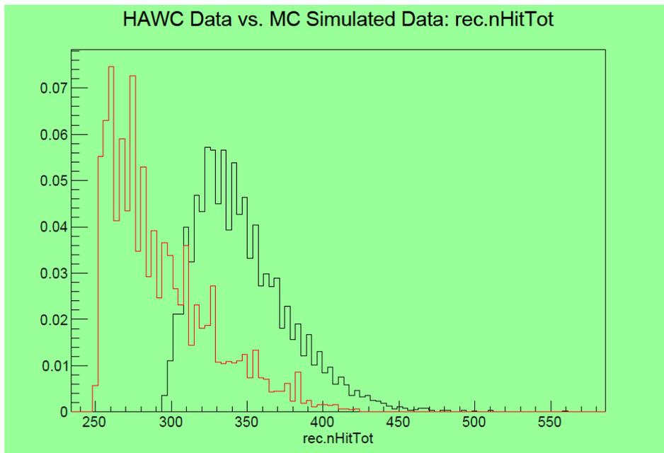
Figure 7: Comparison of total PMTs hit in actual vs. MC data (red = MC, black = actual)
